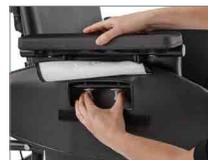
1. Lift flap on outside of armrest to reveal arm height adjustment pins.
